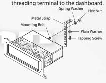
Note: to install the short threading
